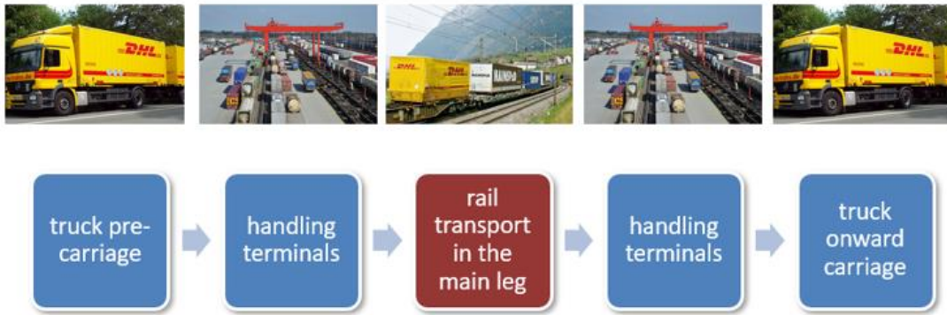
Figure 4: Transport chain in combined transport 12
