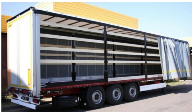
Figure 18: Side-open semi-trailer with sliding tarpaulin
